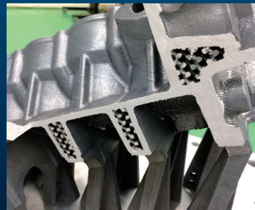
V8 engine block with lattice structure
