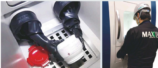
Powder supply (APR system inside)
