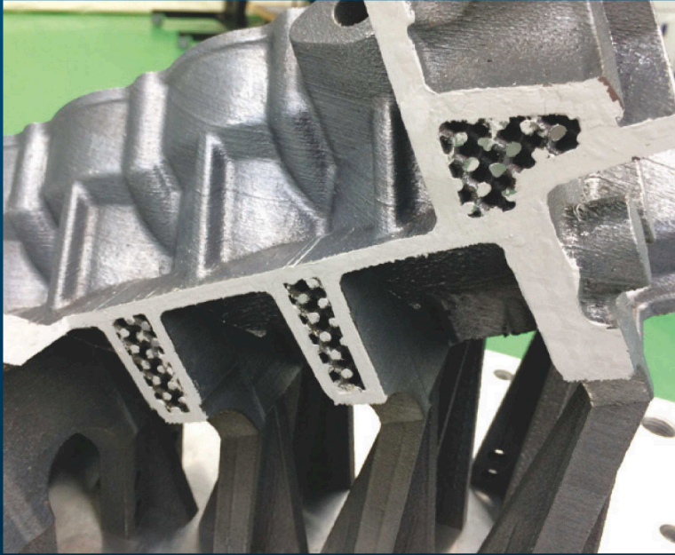
V8 engine block with lattice structure
