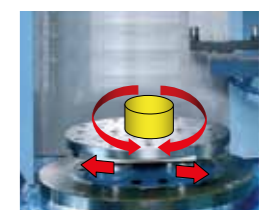
Small inertia (Y-/B-/C-axis and Z-axis optimal acceleration/deceleration)
