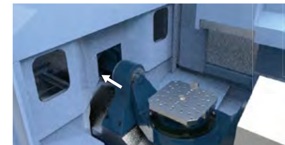
Support retractable under the APC door
