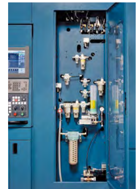
Centralized layout of maintenance devices
