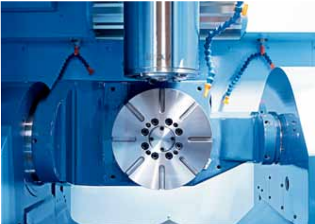
Minimal interference between the spindle head & table, offering excellent workpiece access to the cutting tool.
