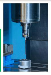
THE RENISHAW OMP400 HIGH ACCURACY PROBE FEATURES AN ULTRA COMPACT DESIGN WITH OPTICAL TRANSMISSION FOR COMPACT TO SMALL MACHINING CENTERS & MILL-TURN CENTERS.
